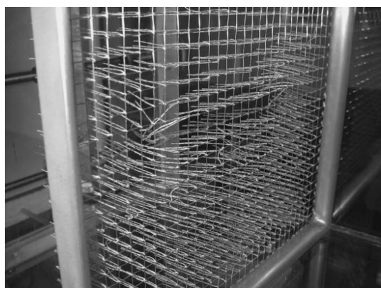
Fig. 11 Tuft grid flow visualization of baseline wing, x/b = 1.0 .
